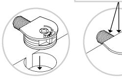
Push a TWIST-LOCK® FASTENER into the large hole in the part.
