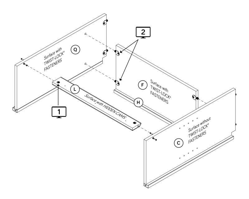
Fasten the SHORT BRACES (N) to the UPRIGHTS (C and Q). Tighten two HIDDEN CAMS.
