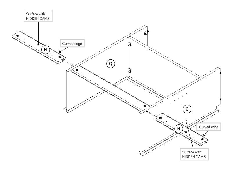
Fasten the ENDS (A and B) to the SHORT BRACES (N). Tighten two HIDDEN CAMS.
