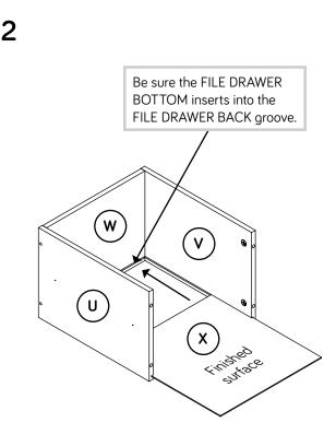
Slide the FILE DRAWER BOTTOM (X) into the grooves in the FILE DRAWER SIDES (U and V) and FILE DRAWER BACK (W).
