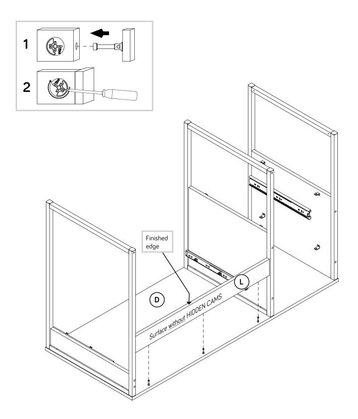
Fasten the SHELF (H) to the UPRIGHT (F) and RIGHT END (G). Use four 7/16" PAN HEAD SCREWS (8) through the METAL BRACKETS (11).
