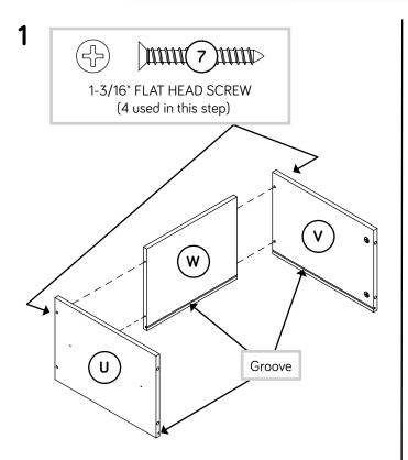
Fasten the FILE DRAWER SIDES (U and V) to the FILE DRAWER BACK (W). Use four 1-3/16" FLAT HEAD SCREWS (7).
