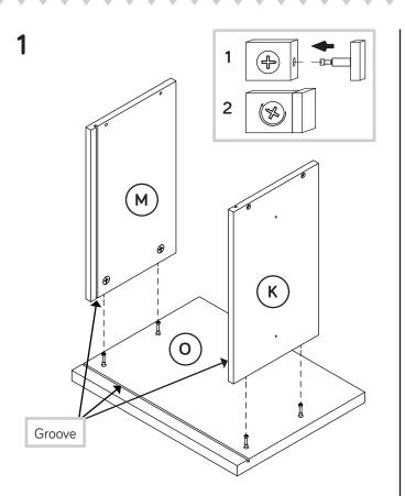
Fasten one each of the DRAWER SIDE (K and M) to a DRAWER FRONT (O). Tighten four HIDDEN CAMS.
