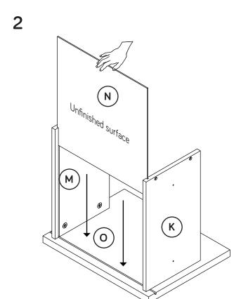
Slide the DRAWER BOTTOM (N) into the grooves in the DRAWER SIDES (K and M) and DRAWER FRONT (O).
