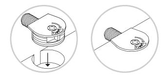
Do <u>not</u> tighten the TWIST-LOCK<sup>®</sup> FASTENERS in this step.
