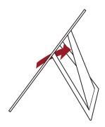
2. Unfold internal rear support leg.
