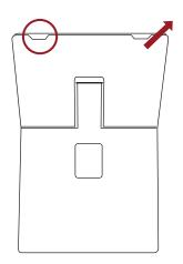
4. Push back plate backwards (finger in cutout) to slightly separate the plates and introduce prop-up of the laptop in between.
