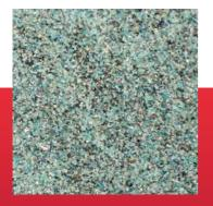
CD and DVDs are shredded in 1,2 x 2 mm small particles
