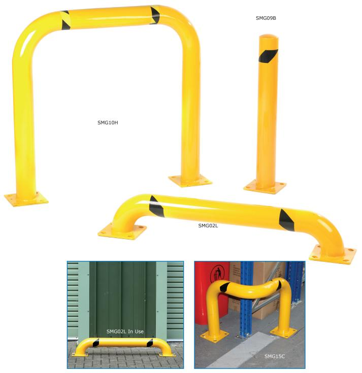
Constructed from heavy duty 115mm diameter steel pipe, these units are ideal for work areas Bases are pre-drilled with 22mm diameter holes for fixing to the floor (not supplied) These units are powder coated yellow for high visibility
