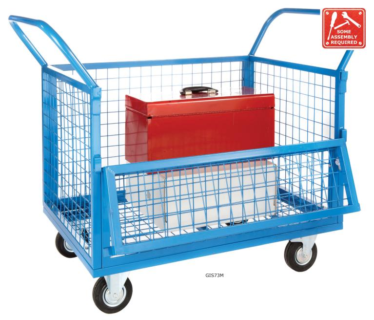
Manufactured from 40mm mesh with a half drop down front Mobile on 2 fixed & 2 swivel braked 200mm castors
