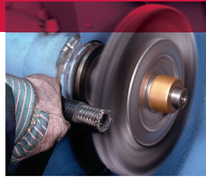
Removing rubber coating from a hydraulic hose.
