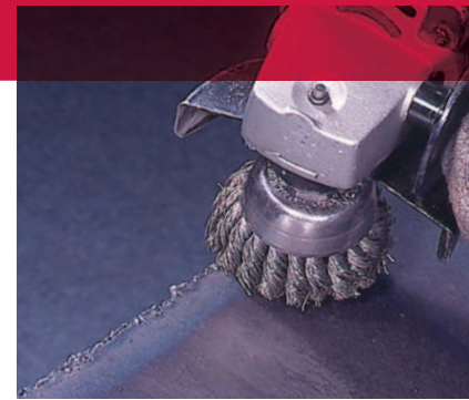
Removing slag from a flame-cut steel plate.
