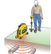
Induce a signal to locate utilities
