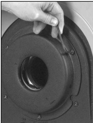
Figure 12A – Removing Rear Chuck Cover
