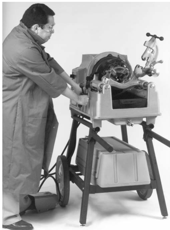
Figure 7 – Threading With 535 Automatic Threading Machine
