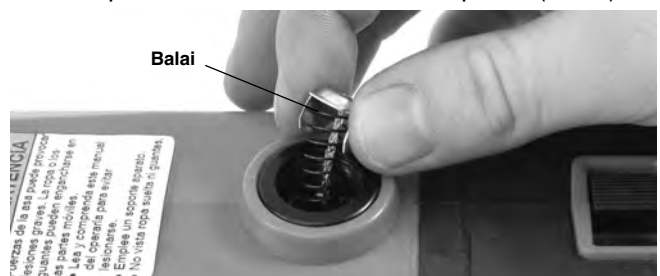
Figure 18 – Installation des balais
