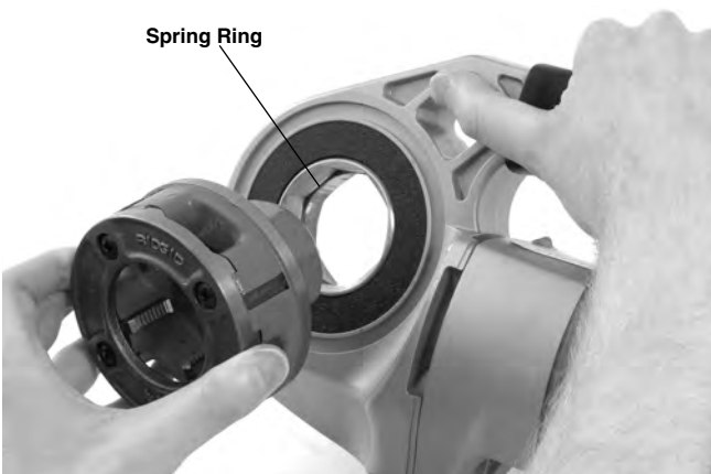
Figure 9 – Installing Die Heads into 600-I Power Drive
