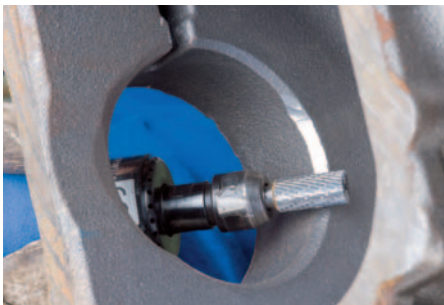
Cylindrical bur with end cut. PFERD specification number ZYAS
