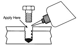
7. Assemble and tighten as usual. When tightening to established torque values, torque compensation is not required.
