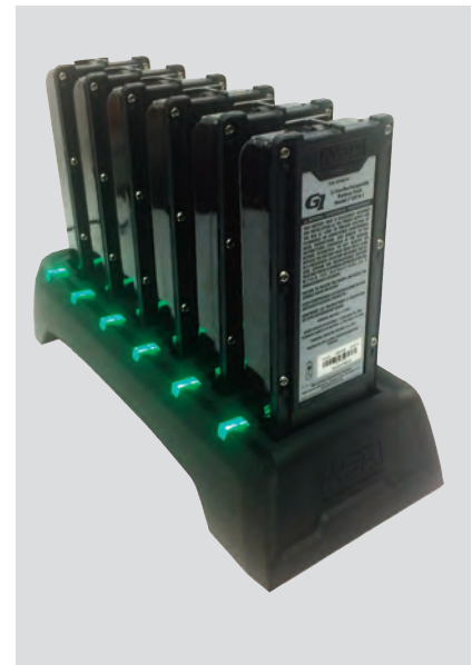
Rechargeable battery packs in battery charging station
