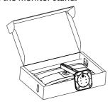
2. While keeping the release button pressed, tilt the base and slide it out.
