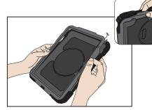
Unlock the clips along the edges to remove the front of the case
