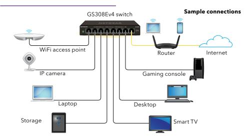
**NOTE:** We recommend that you use a Category 5e (Cat 5e) cable or higher-rated cable for Gigabit Ethernet connections.
