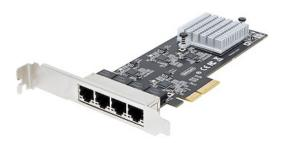
This quad-port 2.5GbE network interface card (NIC) features independent Intel I225-V chipsets for each port with Intel vPro technology, to enhance performance and data integrity across four 2.5G ethernet connections. The variable multispeed options (2.5/1Gbps and 100/10Mbps) enable support for both new and legacy network hardware. Utilize existing Cat5e or CAT6 cabling infrastructure while adding NBASE-T (802.3bz) compatibility for seamless integration.
