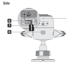
6 microSD Card Slot Insert a microSD card for local recording \*microSD card not included.
