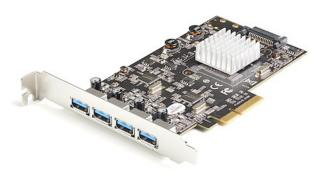
This PCIe USB 3.2 Gen 2 controller card installs into an available PCI-Express x4 slot in your computer and enables you to upgrade your current system by adding four SuperSpeed USB-A (10Gbps) ports. The card features dual ASM3142 controllers with up to 20 Gbps of total bandwidth shared across all 4 ports.
