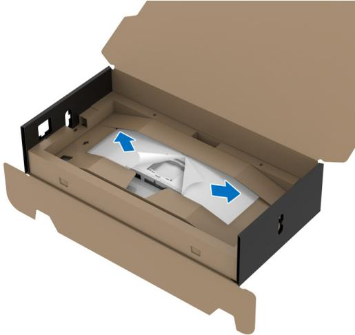
**NOTE:** Before attaching the stand assembly to the display, ensure that the front plate flap is opened to allow space for assembly.
