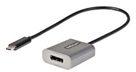
This USB-C to DisplayPort adapter enables you to output DP video and audio from the USB Type-C port on your laptop, tablet, smartphone or other USB C device.
