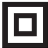
This symbol indicates that this unit is a Class II appliance and therefore an earth connection is not required.
