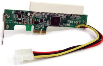
1. Insert the low profile PCI card into the white PCI Slot connector on the top of the adapter card.
