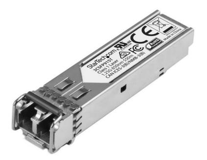
The 3CSFP91ST is an HP 3CSFP91 compatible fiber transceiver module that has been designed, programmed and tested to work with HP® brand switches and routers. It delivers dependable 1 GbE connectivity over fiber cable, for 1000BASE-SX compliant networks, with a maximum distance of up to 550 m (1804 ft).
