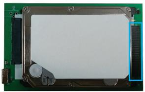
4. Secure the drive in place with the 4 provided drive screws.
