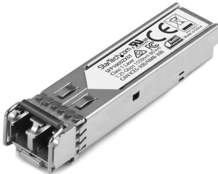
The SFP1000ZXST is an MSA compliant fiber SFP transceiver that's designed, programmed and tested to work with 1000BASE-ZX compatible MSA switches and routers. The SFP transceiver module supports a maximum distance of up to 80 km (49.7 mi) and delivers dependable 1 GbE connectivity over fiber cabling.
