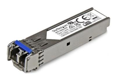
The SFP1000LXST is an MSA compliant fiber SFP transceiver that's designed, programmed and tested to work with 1000BASE-LX compatible MSA switches and routers. The SFP transceiver module supports a maximum distance of up to 10 km (6.2 mi) and delivers dependable 1 GbE connectivity over fiber cabling.
