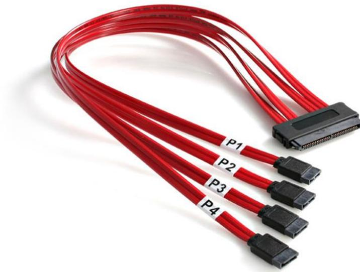
The SAS84S450 SFF-8484 to 4x SATA SAS cable features one 32-pin receptacle (SFF-8484) which fans out to four SATA 7-pin receptacles, providing a reliable solution for connecting up to four SATA HDDs to a SAS controller or backplane.
