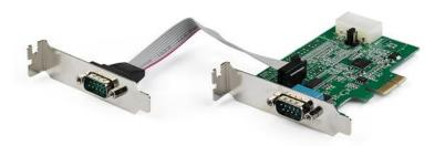
This RS232 Serial Adapter Card lets you add two RS232 (DB9) serial ports to your computer through a PCI Express (PCIe) slot. It enables you to interact with serial devices, such as card readers, printers, PIN pads, and modems, at speeds of up to 921.4Kbps.
