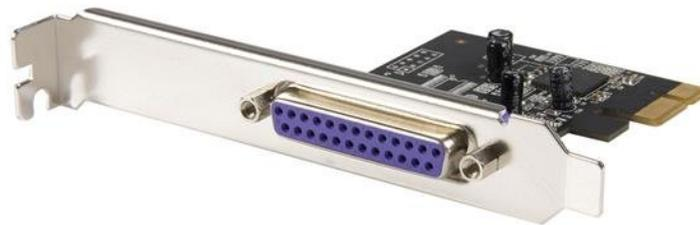
The PEX1P PCIe Parallel Adapter card can be installed in a PCI Express (PCIe) slot, allowing you to connect EPP/ECP parallel peripherals to any computer system. Relying on a native single-chip design(Oxford OXPCIe952), this adapter harnesses the true capability of PCI Express - ensuring maximum performance and reliability.
