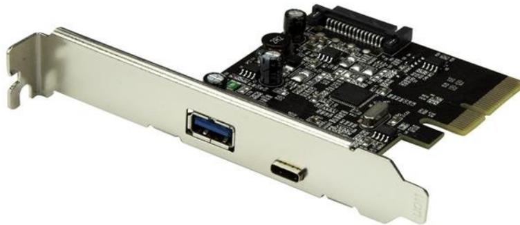
This USB 3.1 card lets you add one USB-C™ port and one USB-A port to your computer, through a PCI Express slot. It enables you to upgrade your current system by adding two USB 3.1 Gen 2 ports to your computer and giving you access to data transfer speeds up to 10Gbps per port.
