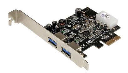
The PEXUSB3S25 2-Port PCI Express USB 3.0 Card lets you add two USB 3.0 ports to your PCI Expressenabled computer system, with an optional LP4 power connector to connect to your system power supply and deliver up to 900mA of power per port to USB 3.0 bus-powered devices (500mA for USB 2.0).
