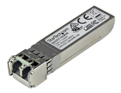
The MASFP10GBSR is a Cisco Meraki MA-SFP-10GB-SR compatible fiber transceiver module that has been designed, programmed and tested to work with Cisco Meraki<sup>™</sup> brand switches and routers. It delivers dependable 10GbE connectivity over fiber cable, for 10GBASE-SR compliant networks, with a maximum distance of up to 300 m (984 ft).
