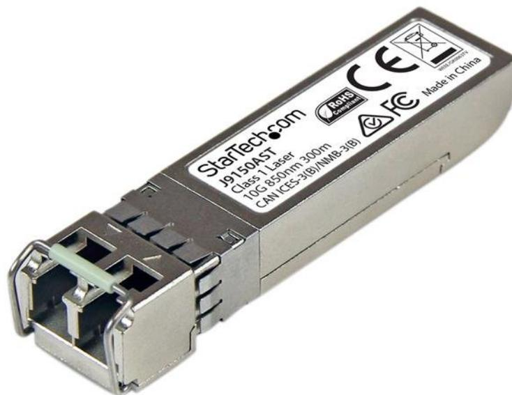
The J9150AST is an HP J9150A compatible fiber transceiver module that has been designed, programmed and tested to work with HP® brand switches and routers. It delivers dependable 10 GbE connectivity over fiber cable, for 10GBASE-SR compliant networks, with a maximum distance of up to 300 m (984 ft).
