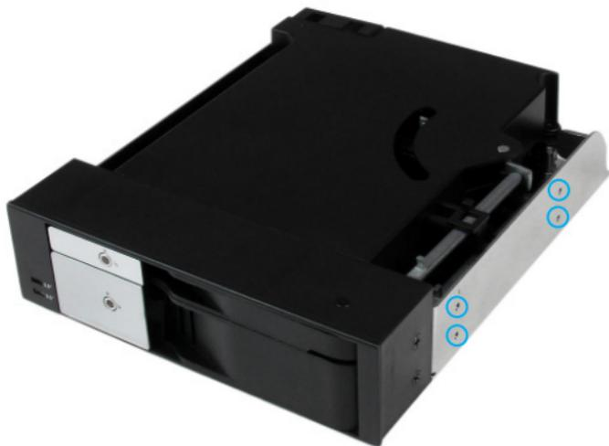
3. Hold the HSB2535SATBK into place, and fix 4 of the included screws through the installation holes on the 5.25" slot, into the side installation holes on the HSB2535SATBK.
