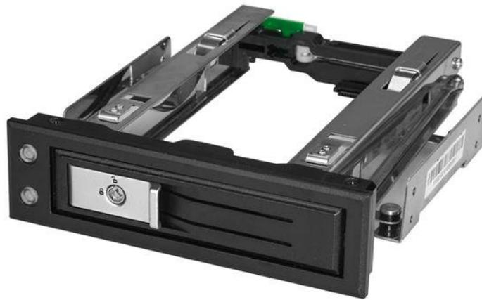
This removable hard drive hot-swap bay makes it easy to swap 3.5" SATA or SAS drives in and out of your server or desktop computer, using an available 5.25" front drive bay. It features a trayless design that saves you installation time and enables you to insert or remove drives as needed. With its durable plastic and aluminum construction, it provides a cost-effective solution for drive maintenance and interchangeability of data between multiple systems.
