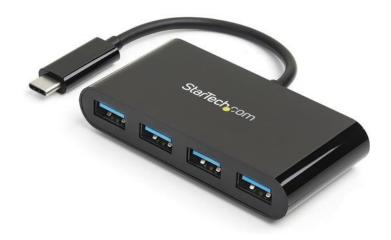
Here's a must-have accessory if you have a USB- $C^{TM}$  equipped computer but need more USB-A ports. This portable USB 3.0 hub expands your laptop or desktop connectivity by adding four USB Type-A ports through a single USB Type- $C^{TM}$  or Thunderbolt<sup>TM</sup> 3 port. And, because it's USB bus-powered, you don't need to connect an external power adapter, which makes travel more convenient and workstations less cluttered.
