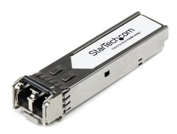
The AR-SFP-1G-LX-ST is an Arista Networks SFP-1G-LX compatible fiber transceiver module that has been designed, programmed and tested to work with Arista Networks brand switches and routers. It delivers dependable 1 GbE connectivity over fiber cable, for 1000Base-LX compliant networks, with a maximum distance of up to 10 km (6.2 mi).
