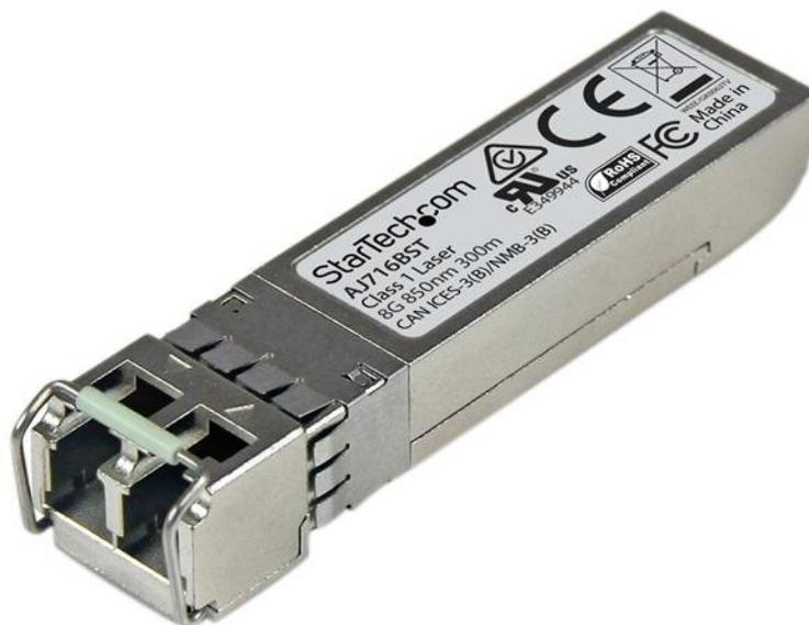
The AJ716BST is an HP AJ716B compatible fiber transceiver module that has been designed, programmed and tested to work with HP® brand switches and routers. It delivers dependable 8Gb fiber channel connectivity over fiber cable, for 8GFC compliant networks, with a maximum distance of up to 300 m (984 ft.).
