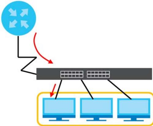
Figure 107 Static Multicast Forwarding to Multiple Ports
