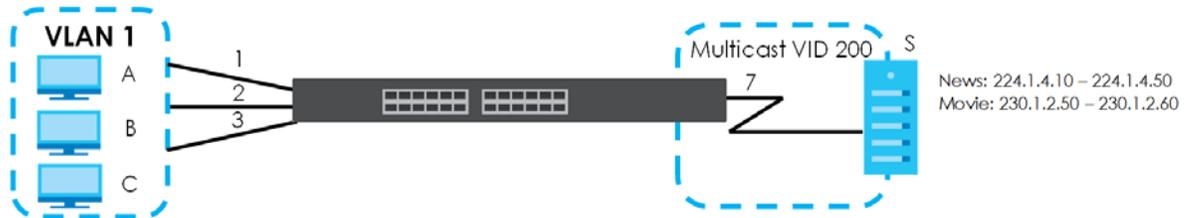
To configure the MVR settings on the Switch, create a multicast VLAN in the **MVR** screen and set the receiver and source ports.
