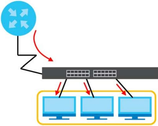
Figure 106 Static Multicast Forwarding to A Single Port
