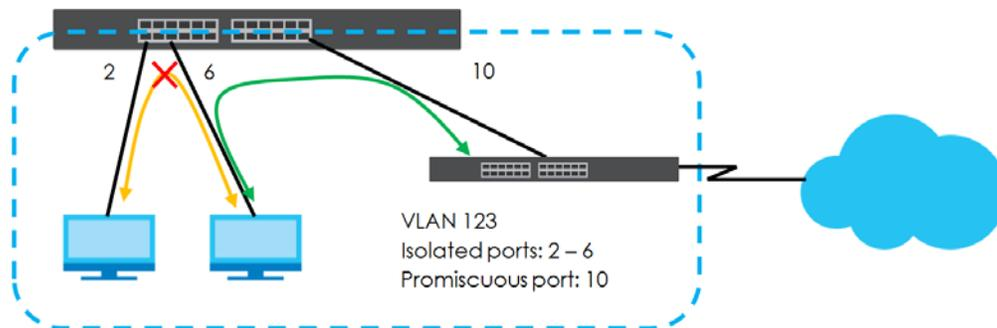
Note: Make sure you keep at least one port in the promiscuous port list for a VLAN with private VLAN enabled. Otherwise, this VLAN is blocked from the whole network.
