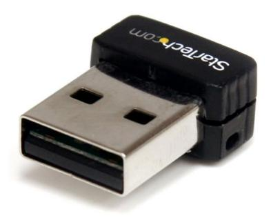
The USB150WN1X1 USB 802.11N Mini Wireless Network Adapter allows almost any USB-enabled desktop, laptop or netbook computer system to connect to 'n', 'g' or 'b' wireless networks. Using a 1T1R (1 Transmitter/1 Receiver) design over the 2.4GHz frequency in an extremely compact form factor, the USB adapter is capable of reaching up to 150Mbps over an 802.11n network while taking up minimal space.
