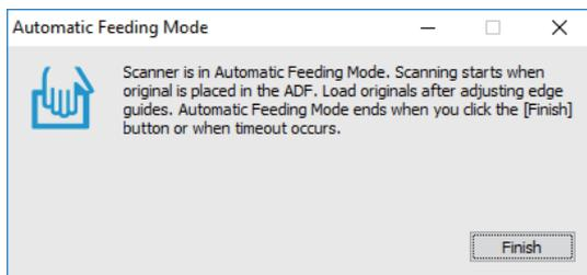
6. Place the original into the scanner until it is fed automatically. Scanning starts automatically.
