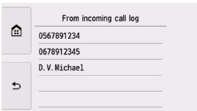
Select a fax/telephone number or name from the incoming call logs, the screen to register the recipient's fax/telephone number and name is displayed. Go to next step.
