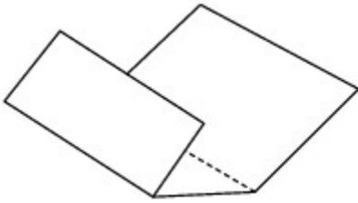
10. Load only this sheet of paper in the cassette with the ridges of the creases facing up and the edge of the half with no crease facing to the far side.
