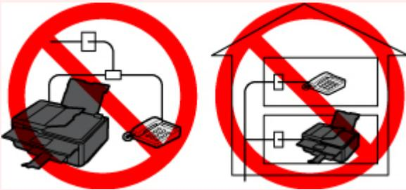
If you cannot avoid parallel connections, set the receive mode to **TEL priority mode**, understanding that the above problems may occur. You will only be able to receive faxes manually.
