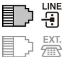
When you connect the telephone to the printer, make sure that the printer is turned off, connect one end of the modular cable to the external device jack near the "EXT." mark of the printer, and then connect the other end to the telephone line jack of the telephone.
