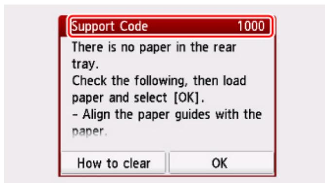
For details on how to resolve errors, see [List of Support Code for Error](#).
