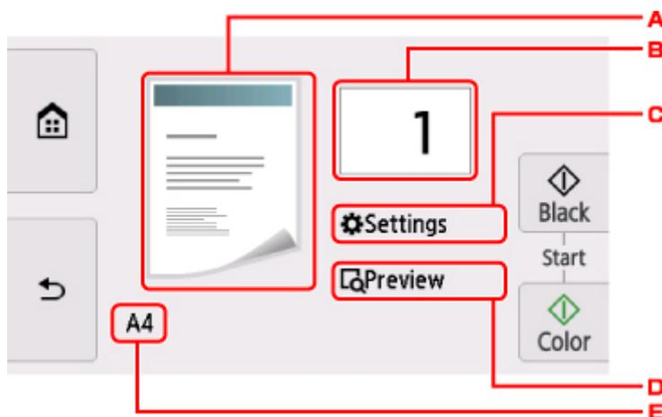
A. The scanning method and copy layout are displayed.
