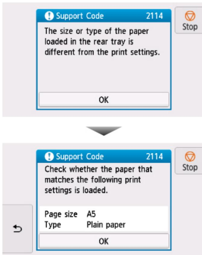
Check the message and select **OK**. When the screen to select the operation is displayed, select one of the operations below.
