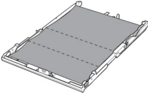
11. Mount the cassette cover, and then insert the cassette into the printer.
