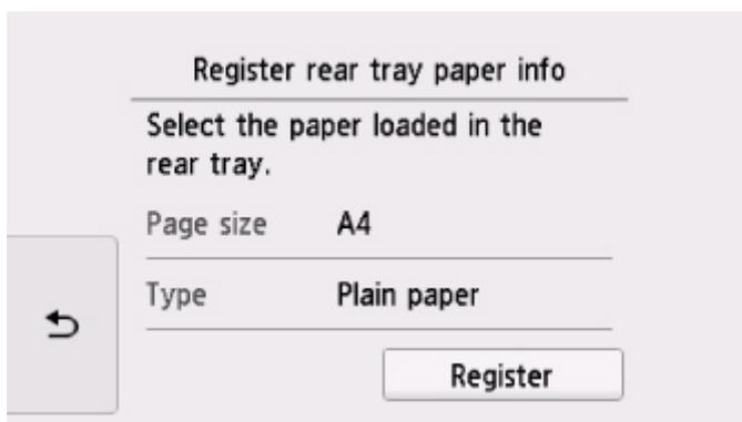
Register the paper size and the media type according to the loaded paper.
