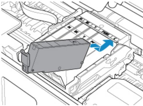
8. Press on the top of the ink tank until the ink tank snaps firmly into place.
