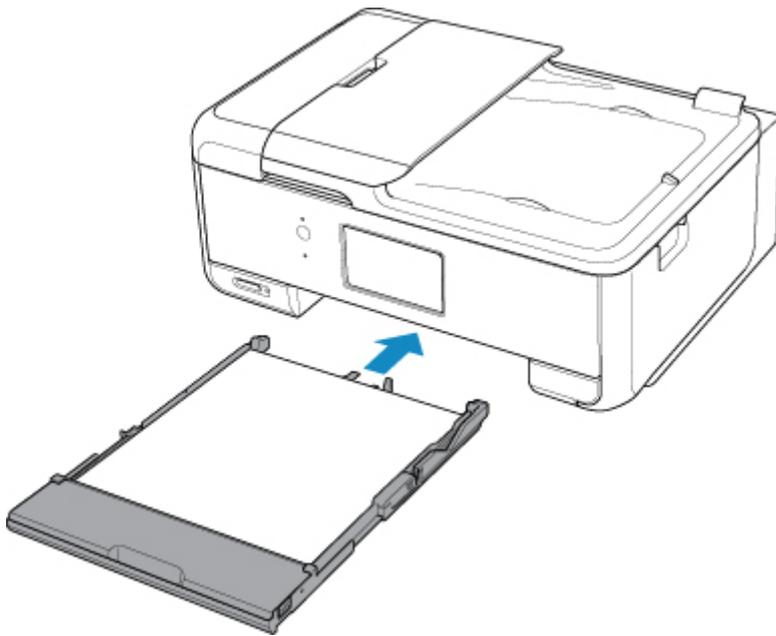
After inserting the cassette into the printer, the paper information registration screen for the cassette is displayed on the touch screen.
