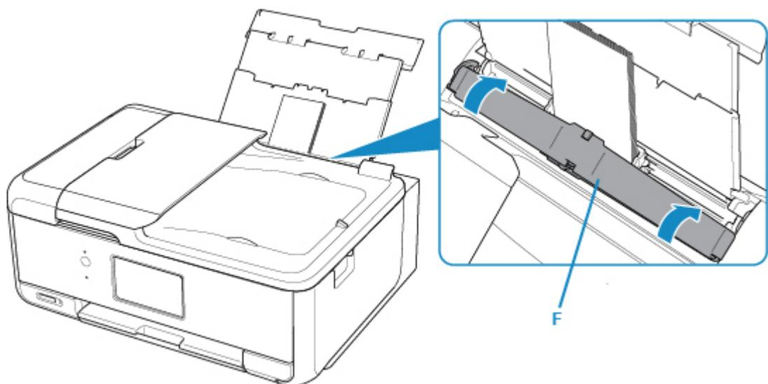
After closing the feed slot cover, the paper information registration screen for the rear tray is displayed on the touch screen.
