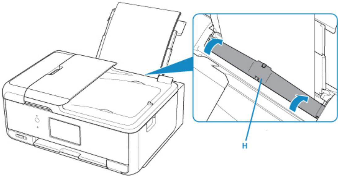
After closing the feed slot cover, the paper information registration screen for the rear tray is displayed on the touch screen.
