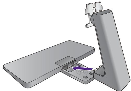
Tighten the thumbscrew on the bottom of the monitor base as illustrated.
