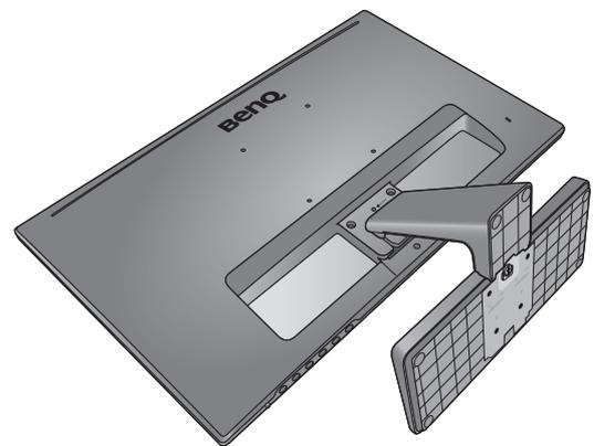
Insert a pointed object such as a screwdriver to the hole above the monitor stand arm, and then push the screwdriver against the release button inside the hole. Then pull the monitor stand backward away from the monitor.
