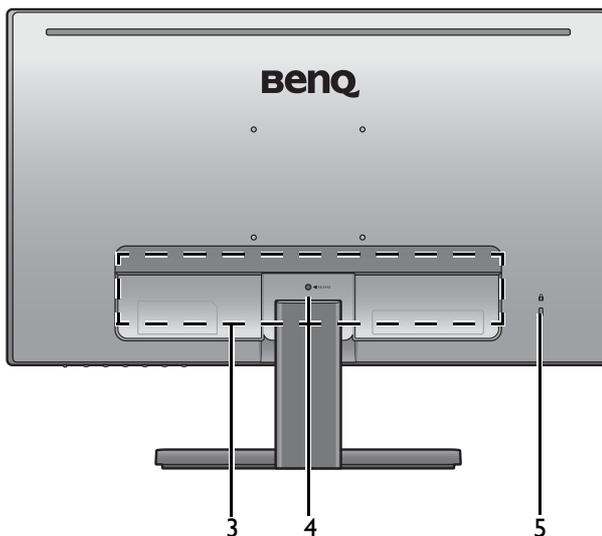
3. Input and output ports (vary by model, see [Input and output ports on page 8](#))
