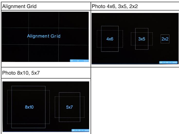
When QuickFit is activated, press the control buttons on the front panel to make adjustments. The QuickFit OSD displayed in the lower right corner of the screen will guide users to make selections.
