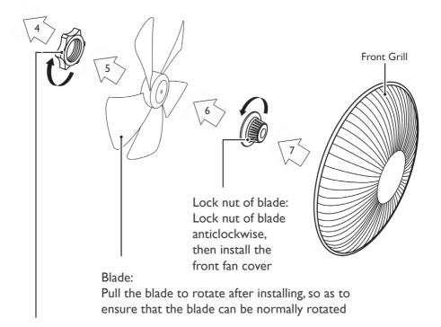
Lock nut of grill: Screw the lock nut of grill clockwise, and ensure the rear grill is kept in place
